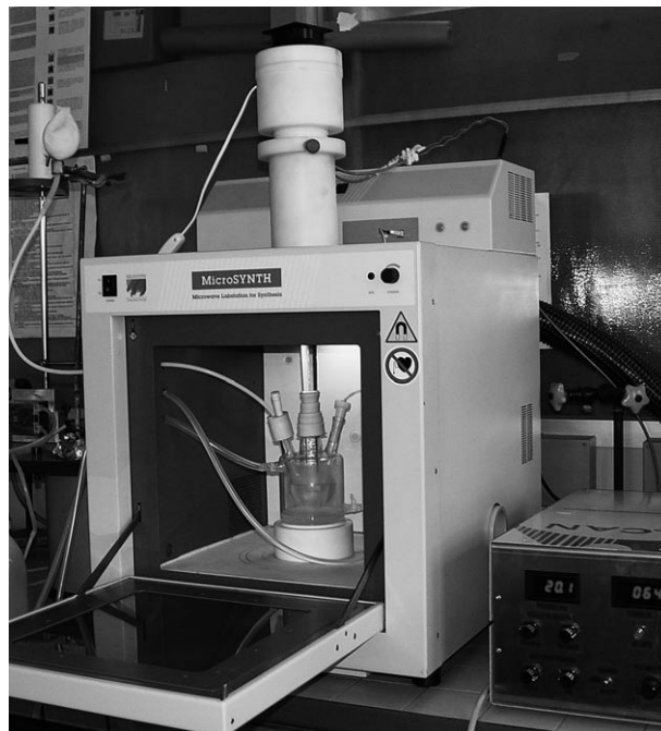
Figure 3. Simultaneous irradiation in a multimode MW oven (Milestone®) equipped with a pyrex horn.
