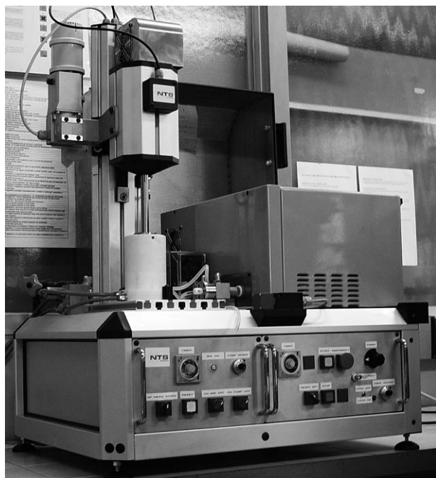
Figure 4. Overall picture of a flow reactor combining MW and US irradiation in a sequential mode.
